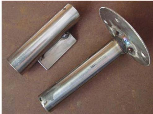
A) Outer holding tube needs to be welded to the frame of the unit (opposite to the CG box) – after removing fiber cover and all the other parts that can interfere with welding process –
